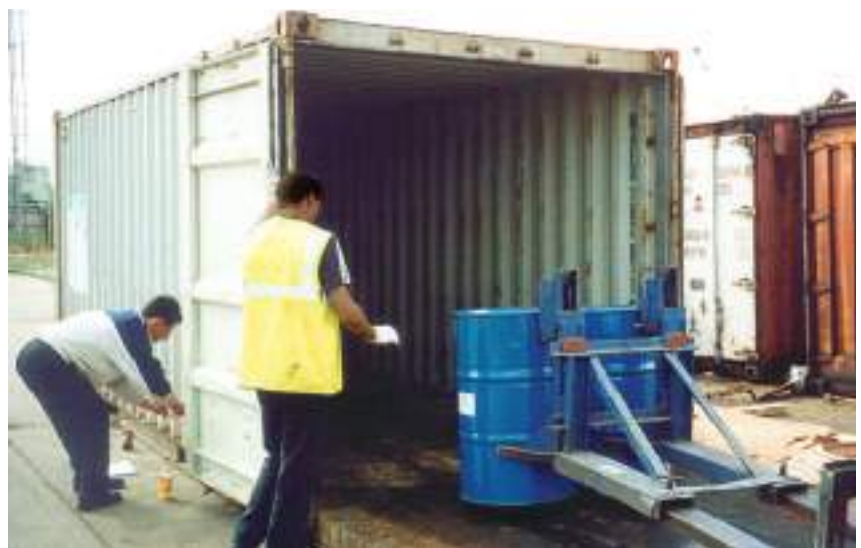
Drums being packed with drum clamps
